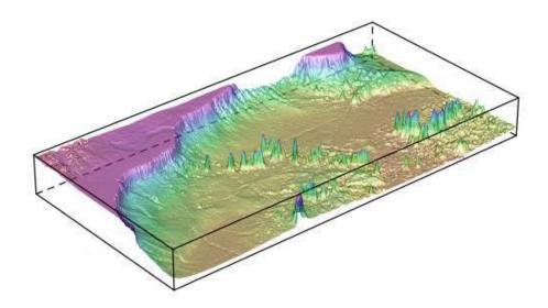
The marmap function get.box() can be coupled with the lattice function wireframe() to produce 3D plots of belt transects of given width. Let's use the NW Atlantic data to investigate these functions, and look at the New England and Corner Rise seamount chains.
