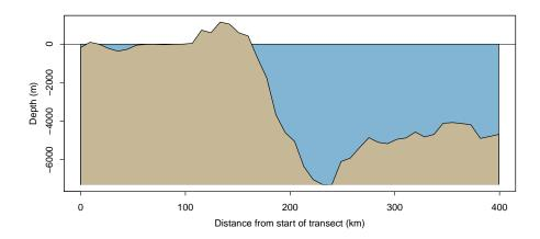
The function path.profile() takes advantage of both get.transect() and plotProfile() to retrieve and plot bathymetric information along a path that is not limited to a straight transect between 2 points. See the help file of plotProfile() for more details.
