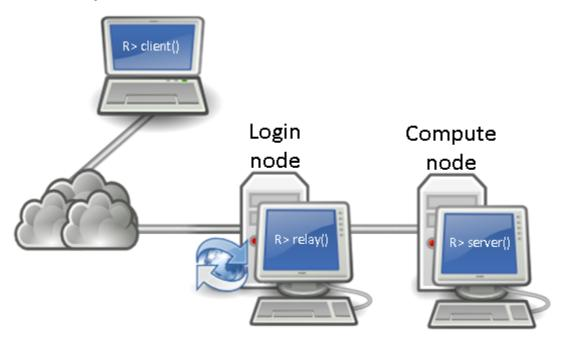
Figure 1: Remoter relays and their relationship to the client and server. The diagram is composed of icons from the OSA Icon Library
